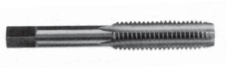
**Plug Taps** - This style, with a **3-5 thread chamfer**, is most widely used in through holes and where there is sufficient room at the bottom in blind holes.
