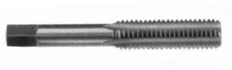
**Bottoming Taps** - This style, designed with a **1 to 2 thread chamfer**, is made with just enough chamfer for starting in the hole; as the name implies, it is designed to thread blind holes to the bottom.
