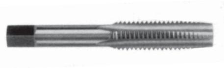
**Taper Taps** - This style, with a **7-10 thread chamfer**, has the longest chamfer of the three to distribute action over the maximum number of teeth; and the taper also acts as a guide in starting the cutting action in the hole. Taper style taps start the thread square with the workpiece. Taper taps are commonly used in through holes and in materials where a tapered guide is necessary.
